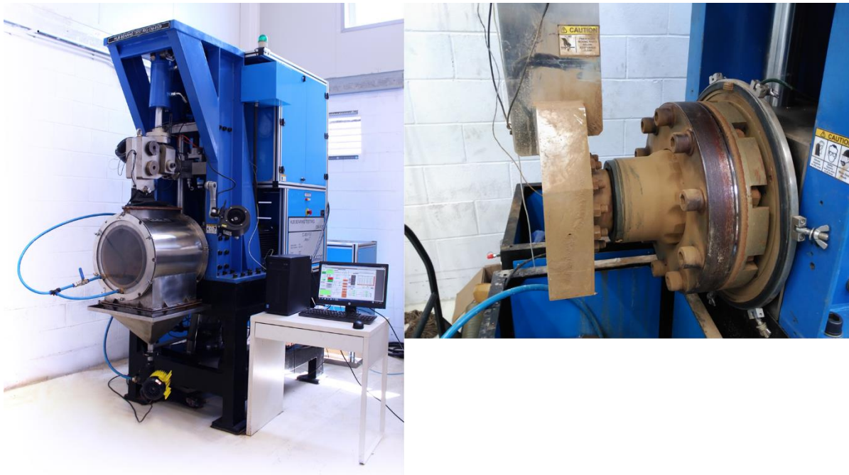
Figure 1. Ducom wheel hub bearing test rig (left) and the wheel hub post submerged test in slurry medium (right). The maximum axial and radial load in this system is 50 kN and 150 kN, respectively. The spindle speed can reach up to 2000 rpm.
